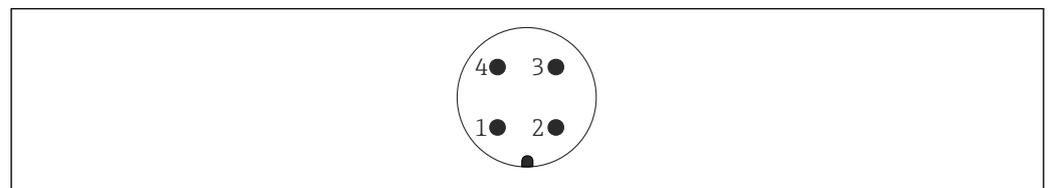
27 Pin assignment of M12 plug
