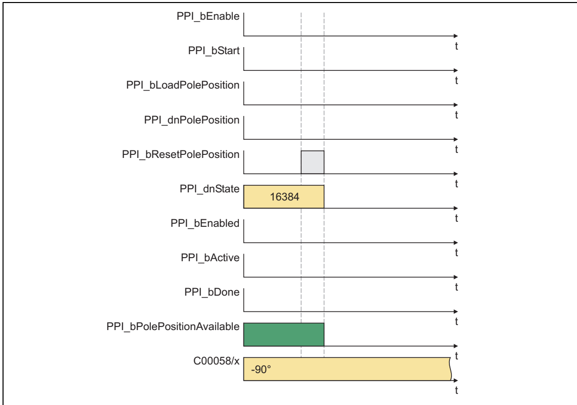
[11-56] Signal characteristic 3: Reset pole position
