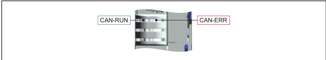
[9-2] LED status displays CAN-RUN and CAN-ERR
