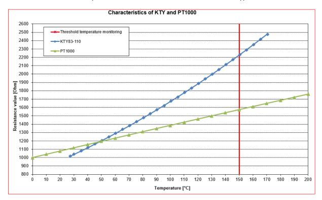
The characteristics are very different from the characteristics of the KTY type used so far.
