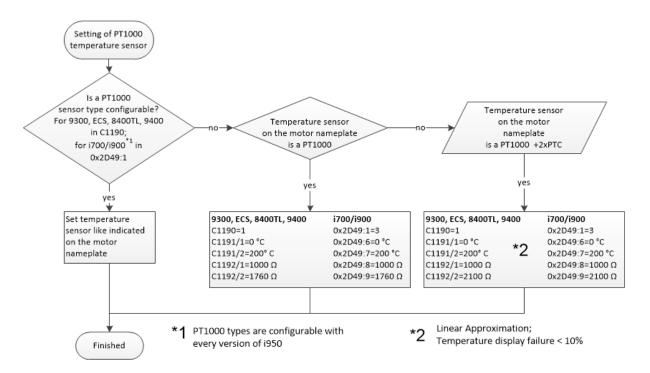
On the motor nameplate, you will find the sensor installed in the motor. During the transitional period, motors equipped with a PT1000 are furthermore provided with a corresponding sticker. In the current servo inverter versions of the 8400TopLine, 9400 HighLine, and the 9400 ServoPLC, the temperature sensor has to be selected as PT1000 or PT1000 + 2xPTC combination in the parameter C1190.
