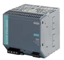
SITOP PSU300S 40A Stabilized power supply input: 3 AC 400-500 V output: 24 V DC/40 A
