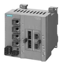
\*\*\*\*\*\*\*\* Replacement part \*\*\*\*\*\*\*\* SCALANCE X308-2M; managed IE switch, compact; 4x 10/100/1000 Mbit/s for RJ45 ports electrical; 2x 100/1000 Mbit/s for 2-port media modules, electrical or optical; LED diagnostics; error signaling Contact; Select/set button; PROFINET IO device; network management; Integrated redundancy manager; office features (RSTP, VLAN, IGMP,...); C-plug in scope of delivery
