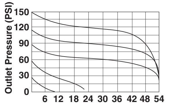
Flow (SCFM) Fig. 6 Valve 40-882-17
