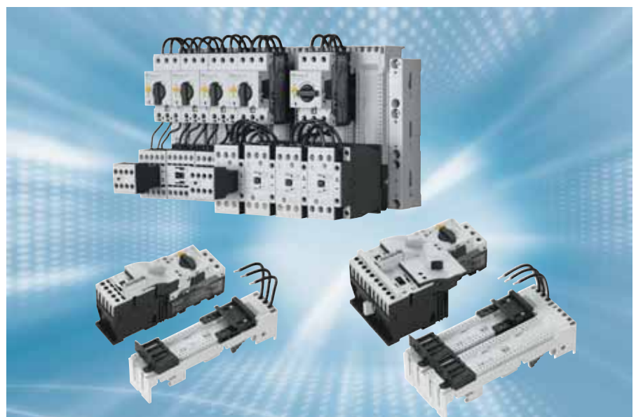
Photo 10: The motor starters as shown in Photo 10 and which are part of a group installation per the NEC/CEC are not required to have the larger distribution clearances. The additional large spacing terminal block is not required in this case. The photo doesn't show the group back-up branch circuit protective device.
