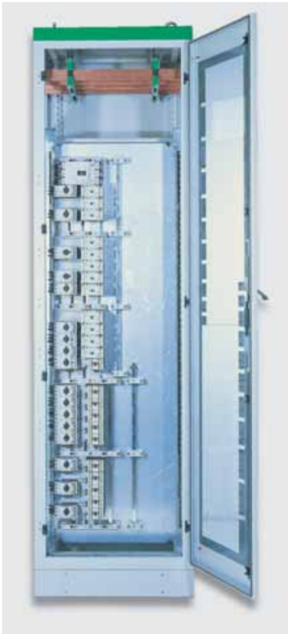
Photo 6: Motor starter section from an engineered product assembly featuring a vertically mounted busbar array to accommodate a large number of motor starters.
