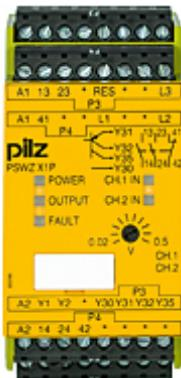
Safety relay (standalone) Inputs: 1-/2-channel wiring. Outputs: 2 N/O, 1 N/C, 2 semiconductor UB 24 - 240 V AC/DC, UM = 0.02 - 0.5 V AC/DC. UMmax = 690 V. Width: 45 mm. Standstill monitor, varnished version The device monitors the EMF voltage created when motors run down.
