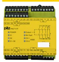
Safety relay (standalone) Inputs: 2-channel wiring with/without detection of shorts across contacts 4 muting sensors. Outputs: 3 2 N/O, 1 N/C, 5 semiconductor. Automatic/monitored start UB 24 V DC, width: 90 mm, plug-in terminals of screw type Device for the temporary suspension of safety functions, muting, monitoring of muting lamps and their automatic switching.
