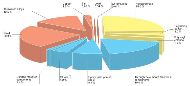
(\*) The "Others" category includes all the elements of which less than 1% was found in the product, such as heat shrink tubing, EPDM elastomer, etc.
