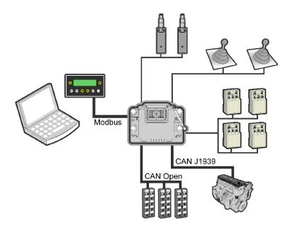
**NOTE:** The different buses must be configured with the TwidoSuite software.
