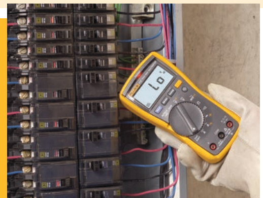
This meter has a built-in non-contact voltage tester.
