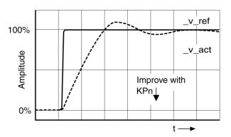
In the case of drive systems in which oscillations occur before the aperiodic limit is reached, the P gain "KPn" must be reduced until oscillations can no longer be detected. This occurs frequently in the case of linear axes with a toothed belt drive.
