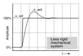
The velocity controller is properly set if the step response is closely resembles the signal illustrated. Good control performance is characterized by
