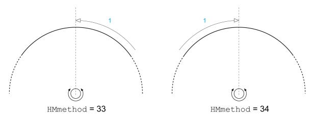
1 Movement to index pulse at velocity HMn\_out
