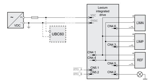
The UBC60 braking resistor controller is available as an accessory, refer to the chapter Accessories and Spare Parts *(see page 253).*
