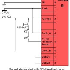
Manual start/restart with EDM feedback loop
