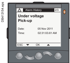
Alarm pick-up and drop-out examples of operating-assistance screens of the FDM121 display unit.
