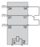
(1) Terminals 11 and 21,14 and 24,12 and 22 must be linked for this references NOTE: For DC input, A1 have to be +, otherwise it would short circuit from protection module
