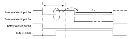
The first safety-related input is deactivated which starts the signal interlock monitoring time of 200 ms. It is then activated again before the second safety-related input is deactivated. This immediately triggers a signal interlock alert even though the 200 ms have not yet elapsed.
