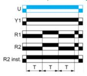
Function DW: Symmetrical Flashing Relay (Starting Pulse Off) & With Retrigger / Restart Control
