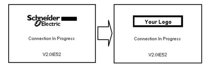
From the firmware version V2.0 of the Graphic Display Terminal, the logo displayed at power on by the Graphic Display Terminal can be customized. By default, the Schneider-Electric logo is displayed.
