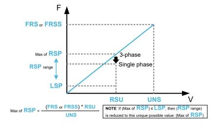
**NOTE:** Compared to a 3–phase power backup supply, the **[Pwr Backup Ref Freq]** r 5 P value may need to be reduced in order to provide the nominal torque with a single phase power backup supply. For more information, you must refer to the application note "Power Backup".
