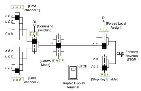
[Cmd channel 1] [ d I and [Cmd channel 2] [ d 2: Terminals, Display Terminal, integrated Modbus, integrated CANopen®, communication card
