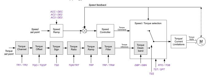
The function can be used to switch between operation in speed regulation mode and operation in torque control mode.
