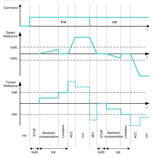
Regulate 0Hz speed at direction change (UC-3)
