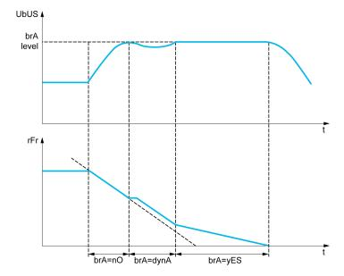
Activating this function automatically adapts the deceleration ramp, if this has been set at a too low value according to the inertia of the load, which can cause an overvoltage detected error.
