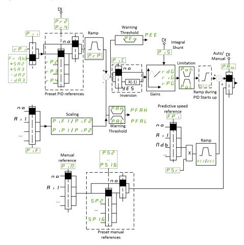
The PID feedback needs to be assigned to one of the analog inputs AI1 to AI5 or a pulse input, according to whether any I/O extension module has been inserted.
