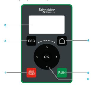
1 STOP / RESET: Stop command / apply a Fault Reset.
