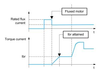
When run command is given, the drive over-fluxes the motor during a short time in order to generate a sufficient motor torque. The level of the torque is set with the parameter **[Brk Release Current]** , b r. This torque is required to maintain the load during the release of the brake and before starting speed control.
