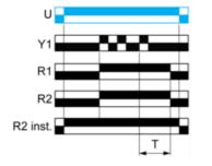
Function O : Delayed Safe-Guard Relay
