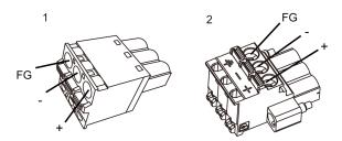
1 Straight type: HMIZGPWS by Schneider Electric
