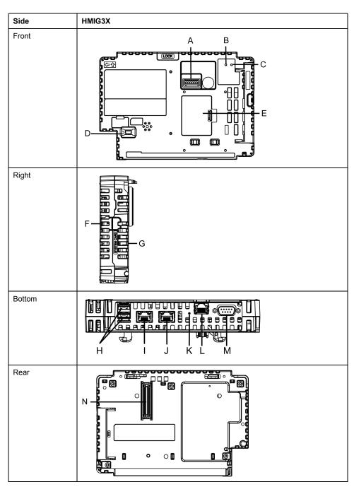
A: Auxiliary output/ Speaker output interface (AUX)
