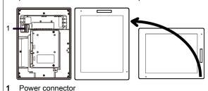
When installing this product in a slanted position, the product face should not incline more than 30°.
