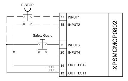
Type C, class 3 according to "ZVEI CB24I Ed.2" with a maximum test pulse duration of 100 µs.
