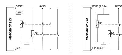
Dual channel OSSD configuration with 2 dual channel Single channel OSSD configuration with 4 single outputs, safety category SIL3/PL e: EN 61508:2010
