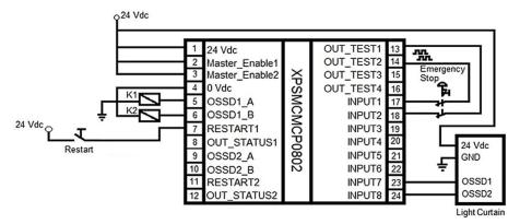
**NOTE:** Best practice dictates the use of fusing on the incoming 24 Vdc power, and sized appropriately for the requirements of the module.
