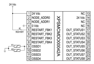
**NOTE:** Best practice dictates the use of fusing on the incoming 24 Vdc power, and sized appropriately for the requirements of the module.
