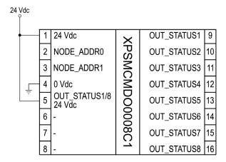
**NOTE:** Best practice dictates the use of fusing on the incoming 24 Vdc power, and sized appropriately for the requirements of the module.
