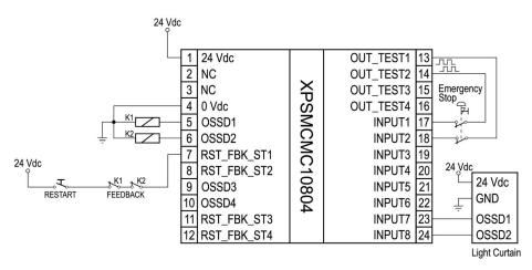
**NOTE:** Best practice dictates the use of fusing on the incoming 24 Vdc power, and sized appropriately for the requirements of the module.
