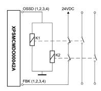
Dual channel OSSD configuration with 2 dual channel outputs, safety category SIL3/PL e: EN 61508:2010
