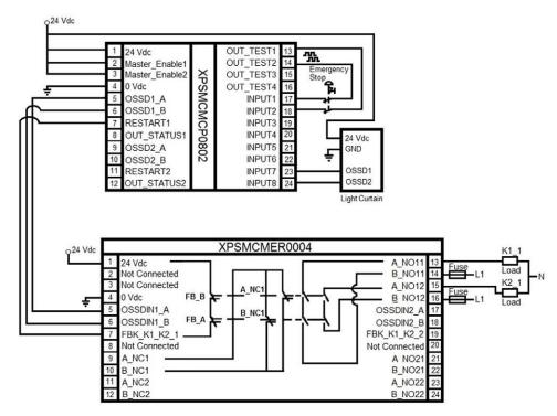
**NOTE:** Best practice dictates the use of fusing on the incoming 24 Vdc power, and sized appropriately for the requirements of the module.
