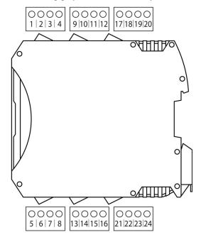
The terminal blocks are either screw or spring cage clamp terminal blocks depending on the reference.
