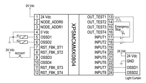
NOTE: Best practice dictates the use of fusing on the incoming 24 Vdc power, and sized appropriately for the requirements of the module.
