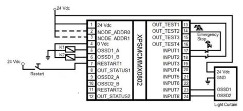
**NOTE:** Best practice dictates the use of fusing on the incoming 24 Vdc power, and sized appropriately for the requirements of the module.
