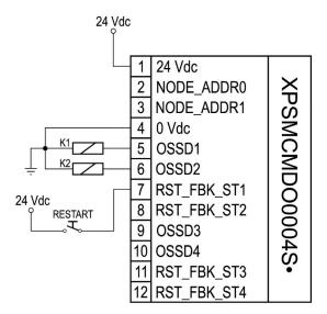
**NOTE:** Best practice dictates the use of fusing on the incoming 24 Vdc power, and sized appropriately for the requirements of the module.
