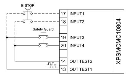
Type C, class 3 according to "ZVEI CB24I Ed.2" with a maximum test pulse duration of 100 µs.
