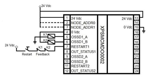
**NOTE:** Best practice dictates the use of fusing on the incoming 24 Vdc power, and sized appropriately for the requirements of the module.
