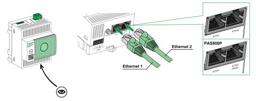
**NOTE**: PAS800P can be powered by Power over Ethernet (PoE). For information about connection of PAS800P to an Ethernet switch with Endspan PoE ports or Midspan PoE ports, consult the instruction sheet available on the Schneider Electric website: JYT24469 *EcoStruxure Panel Server Advanced - Instruction Sheet*.
