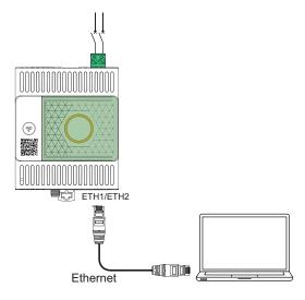
To connect a PC to EcoStruxure Panel Server through Ethernet, connect an Ethernet cable between the PC and one of the Ethernet ports on the EcoStruxure Panel Server (ETH1 or ETH2).
