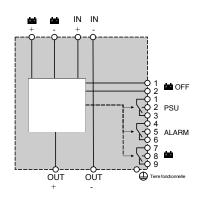
Regulated switch mode power supplies Function modules (for Universal range): Redundancy module
