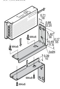
Plate-mounting using the ABL1A02 clip-on plate on a 35 mm DIN rail
