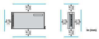
In all cases, there must be adequate convection around the products to help ensure sufficient cooling. There must be a clear space of 1.97 in (50 mm) above and below the power supplies, and of 0.79 in (20 mm) at the sides.
