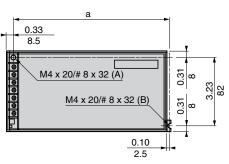
Back-of-cabinet mounting using the ABL1A01 reversible bracket with 3  $\boxtimes$  4 mm screws
