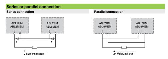
1 Two shottky diodes, Imin = power supply In, and Vmin = 50 V
