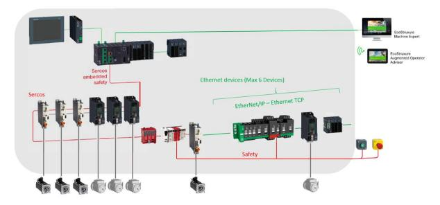
An additional gateway is not required. Configuration is performed in EcoStruxure Machine Expert. Place the Ethernet device after the last Sercos device. The last Sercos device is used as a gateway. It must provide two Sercos connectors.
