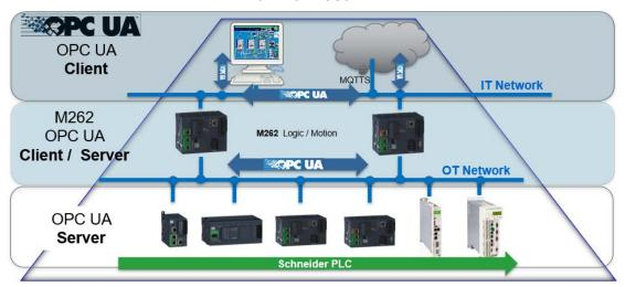
OPC UA data exchange is performed using function blocks that are compliant with the PLCopen specification *PLCopen OPC-UA Client for IEC61131-3 version 1.1* and provide the following functions:
