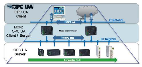
OPC UA data exchange is performed using function blocks that are compliant with the PLCopen specification *PLCopen OPC-UA Client for IEC61131-3* version 1.1 and provide the following functions:
