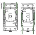
Pluggable auxiliary contact, OF or SD dependent on cavity. Multiple internal wiring possibilities, even with long terminal shields
