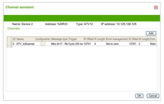
Preconfigured channels are displayed with a lock symbol and a gray background. Some parameters cannot be modified for predefined channels.
