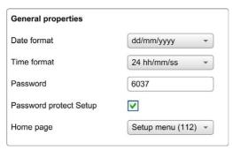
You may select time and date formats, the home page for the Operator Interface that you have defined, and the password used for the Remote Graphic Display. The password is effective in helping to protect the Operator pages that you have selected to be protected, and, if you choose, the Setup pages that affect the logic controller state and data.
