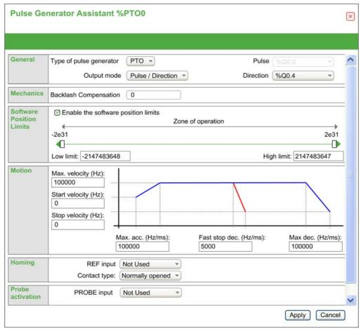
The table describes each parameter available when the channel is configured in PTO mode:
