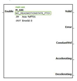
**NOTE:** When you first enter the function block, you must configure it to use the intended axis. Double-click on the function block to display the function block properties, choose the axis and click Apply.
