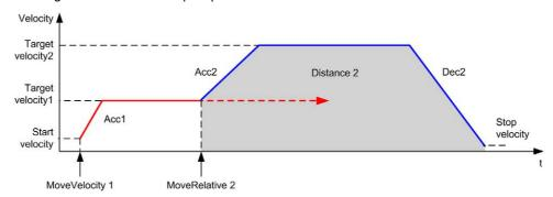
The diagram illustrates a complex profile from **Continuous** state with change of direction:
