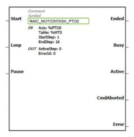
**NOTE:** When you first enter the function block, you must configure it to use the intended axis and motion task table. Double-click the function block to display the function block properties, choose the axis and table, then click Apply.
