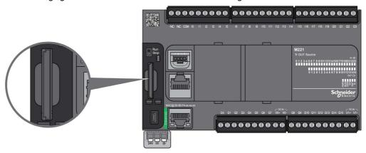
The following figure shows the SD card slot of the TM221M Logic Controller:
