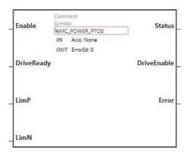
**NOTE:** When you first enter the function block, you must configure it to use the intended axis. Double-click on the function block to display the function block properties, choose the axis and click Apply.
