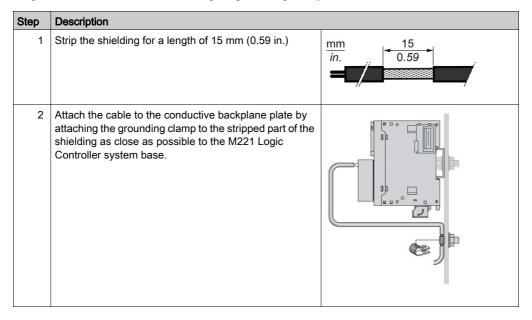
**NOTE:** The shielding must be clamped securely to the conductive backplane to ensure a good contact.
