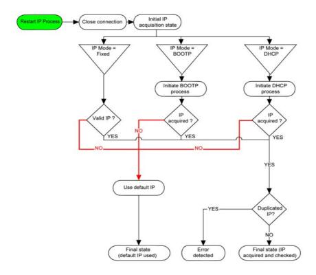
**NOTE:** If a device programmed to use the DHCP or BOOTP addressing methods is unable to contact its respective server, the controller uses the default IP address. It will, however, constantly repeat its request.
