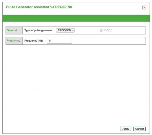
The Frequency Generator (FG) function generates a square wave signal with programmable frequency and duty cycle of 50%. The controller uses an internal clock generator and provides an output signal on a dedicated output channel (%Q0.0). This output signal can directly command a constant motion of the axis. The target frequency is always positive.
