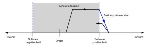
**NOTE:** In previous diagram, the axis move back in the limits is the result of the execution of MC\_Reset\_PTO (it is not performed automatically).
