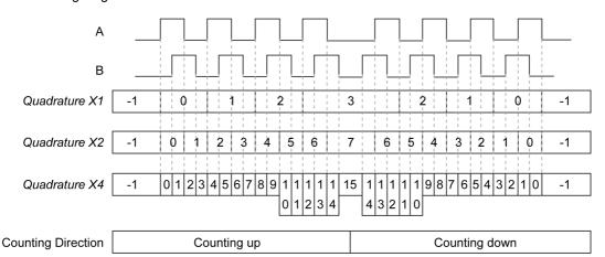
**Quadrature X1** When channel A leads channel B, the counter increments on the rising edge of channel A. When channel B leads channel A, the counter decrements on the falling edge of channel A.
