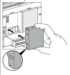
5 Push the cartridge slot cover into the slot until it clicks.
