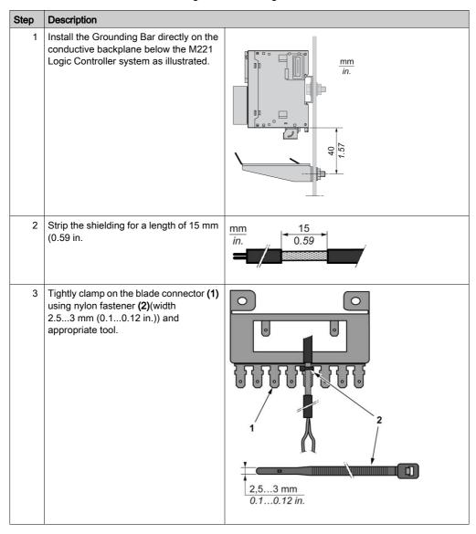
NOTE: Use the TM2XMTGB Grounding Bar exclusively for Functional Ground (FE) connections.
