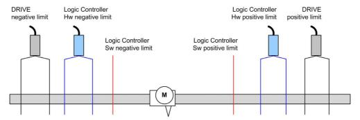
Once either the controller hardware or software limits are crossed, an error is detected and a Fast stop deceleration is performed:
