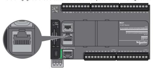
The following figure shows the location of the serial line 1 port on the TM221M Logic Controller:
