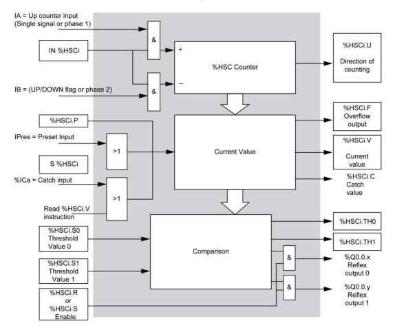
**NOTE:** Reflex outputs are managed independently from the controller cycle time.
