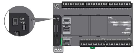
The following figure shows the location of the Run/Stop switch on the TM221M Logic Controller:
