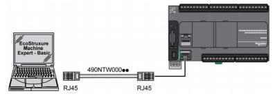
The following illustration shows the Ethernet connection to a PC on a TM221M Logic Controller:
