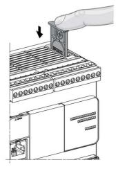
Slide in the battery holder of the TM221M Logic Controller.
