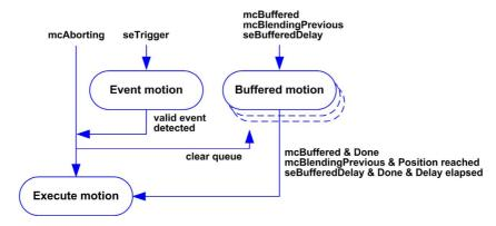
The buffer can contain only one motion function block.
