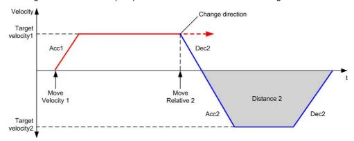
The diagram illustrates a complex profile from **Discrete** state:
