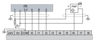
TM221C••R / TM221CE••R with a dual-phase encoder with index and PNP sensor:
