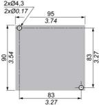
The following diagram shows the mounting hole layout for TM221C Logic Controller with 24 I/O channels:
