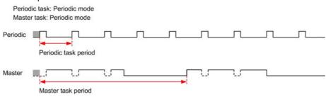
If the processor goes to the HALTED state when the master task is configured in freewheeling mode, verify whether the periodic task scan delay time is significant in comparison to the periodic task period. If so, try:
