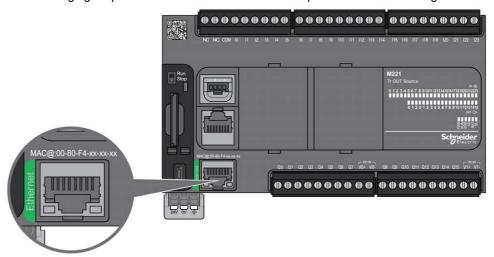
The following figure presents the location of the Ethernet port on the TM221M Logic Controller:
