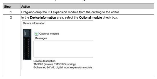
To mark an existing I/O expansion module as optional in the configuration:
