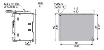
The following diagram shows the mounting hole layout for TM221C Logic Controller with 40 I/O channels:
