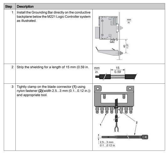
NOTE: Use the TM2XMTGB Grounding Bar exclusively for Functional Ground (FE) connections.
