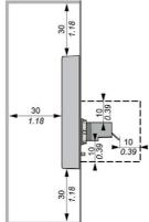
**NOTE:** Keep adequate spacing for proper ventilation and to maintain the operating temperature specified in the Environmental Characteristics (see page 16).
