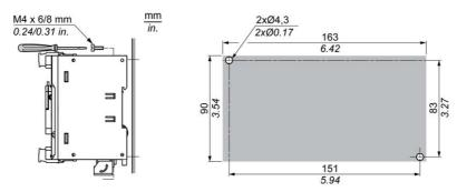
The following diagram shows the mounting hole layout for TM221M Logic Controller:
