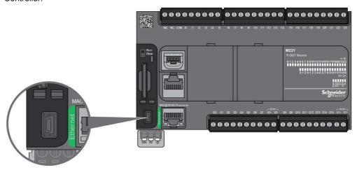
The following figure shows the location of the USB Mini-B programming port on the TM221M Logic Controller:
