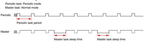
In freewheeling mode, the master task sleep time is at least 30% of the total cycle time with a minimum of 1 millisecond. This percentage may be higher depending on the user application (periodic task scan time, event task scan time, communication interaction, and so on).
