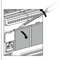
4 Remove by hand the cartridge slot cover from the controller.
