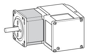
The Lexium integrated drive consists of a stepper motor and an integrated drive. The product integrates interfaces, control electronics, a holding brake (optional) and the power stage.
