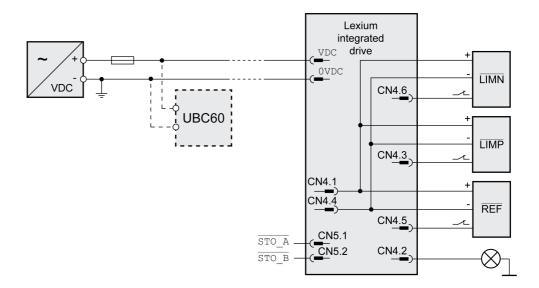
The UBC60 braking resistor controller is available as an accessory, refer to the chapter Accessories and Spare Parts *(see page 225).*
