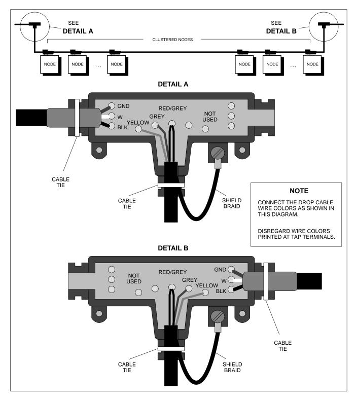
Figure 8 Connecting the Drop Cable to the Tap
