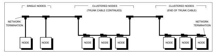
Figure 1 Overview: Network with Single Nodes and Clustered Nodes
