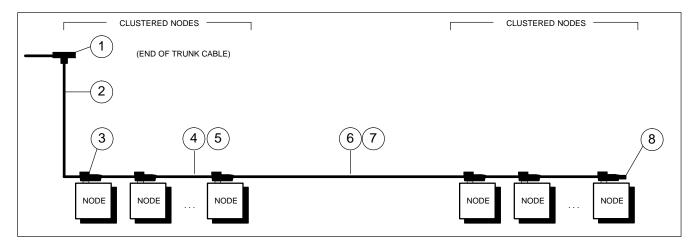
Figure 3 Cluster Configuration: End of Trunk Cable
