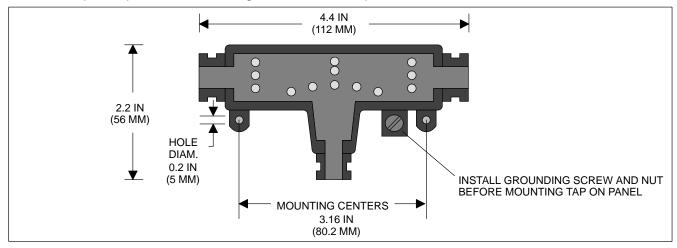
Install the Tap at its planned location. Figure 5 shows the Tap's dimensions.
