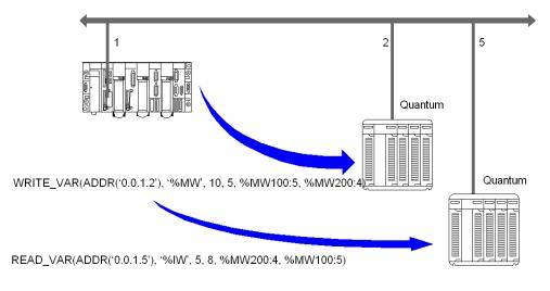
The internal words to write to station 2 are located at address 10. The input words to read from station 5 are located at address 5.
