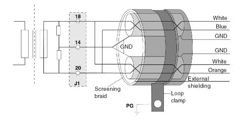
**NOTE: Important**: The cable's main shielding is grounded using a metal clamp in contact with the screening braid, which itself is fixed to the frame supporting the rack. This cable must be grounded, even if there is no PCMCIA card present.
