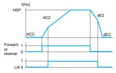
Acceleration 1 (ACC) and deceleration 1 (dEC): -Adjustment 0.1 to 999.9 s
