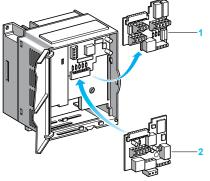
Example of installation of a communication card (1)
