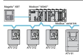
Example of configuration on Modbus serial link
