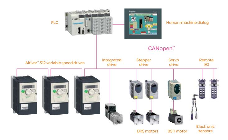
Altivar<sup>™</sup> 312 drives integrate transparently into your architectures and communicate with most control system products:
