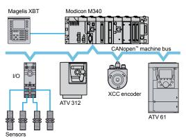
Example of configuration on CANopen machine bus
