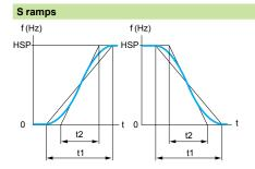
HSP: high speed t1: ramp time set  $t2 = 0.6 \times t1$ The rounding coefficient is mounted. U ramps f (Hz) f (Hz) HSP HSF 0 t2 t2
