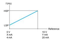
LSP: low speed, from 0 to HSP, factory setting 0 HSP: high speed, from LSP to f max., factory setting 50 Hz
