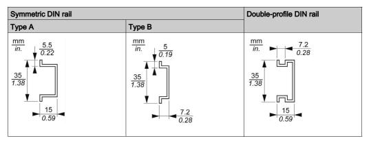
NOTE: When mounted on a type B symmetric DIN rail, the rack withstands less mechanical stress.
