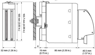
a DIN-rail depth: the value depends on the DIN-rail type used in your platform.
