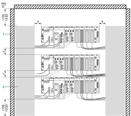
This illustration shows the rules of an installation in a cabinet without horizontal ducts between two racks:
