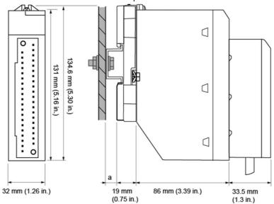
a DIN-rail depth: the value depends on the DIN-rail type used in your platform. Refer to Mounting the Racks (see page 39).
