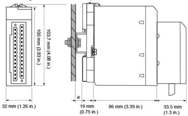
**a** DIN-rail depth: the value depends on the DIN-rail type used in your platform. Refer to *Mounting the Racks* (see page 39).
