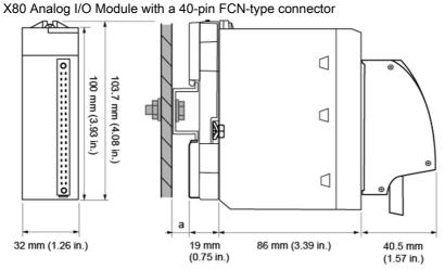
a DIN-rail depth: the value depends on the DIN-rail type used in your platform.
