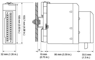
a DIN-rail depth: the value depends on the DIN-rail type used in your platform.
