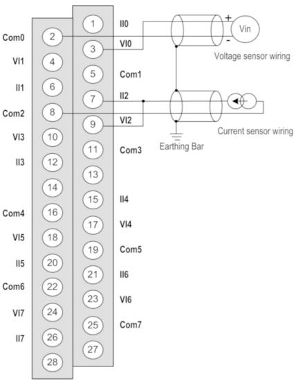
VIx + pole input for channel x COM x - pole input for channel x IIx current reading resistor + input Channel 0 voltage sensor Channel 1 2-wire current sensor
