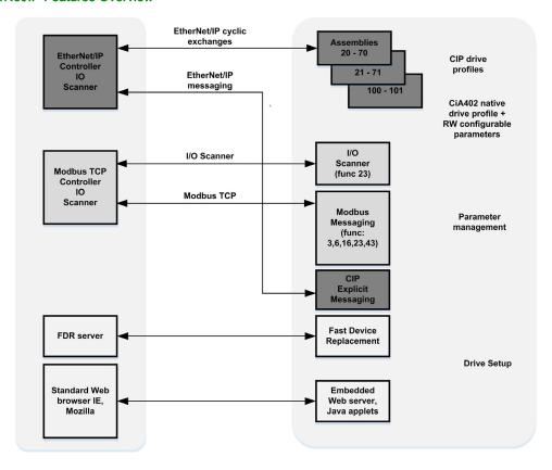
**NOTE:** When using ModbusTCP, it is advisable to use function codes 16 or 23 to control the drive.
