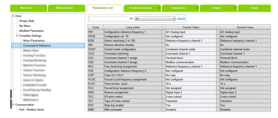
• Configure [Ref Freq 1 Config] F r I parameter to [Embedded Ethernet] E L H value.
