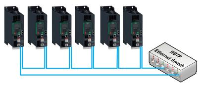
• Redundant ring topology with RSTP (with a RSTP PLC)
