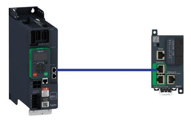
The drive is controlled from the communication but the frequence reference value is adjusted with analog input 1. The control word comes from the controller and is written according to CiA 402 profile.
