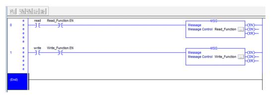
The Read Boolean will trigger the Read Function to read the # [ parameter.
