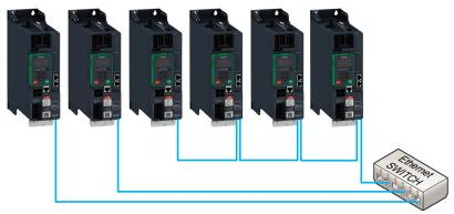
**NOTE:** In daisy chain topology, if one drive is turned off, an **[Embd Eth Com Interrupt]** *E E H F* error is trigged in the other drives connected to the same topology. To keep the integrity of Ethernet daisy chain network when one or more drives are powered off, add an external permanent 24VDc supply to the control block of the drive.
