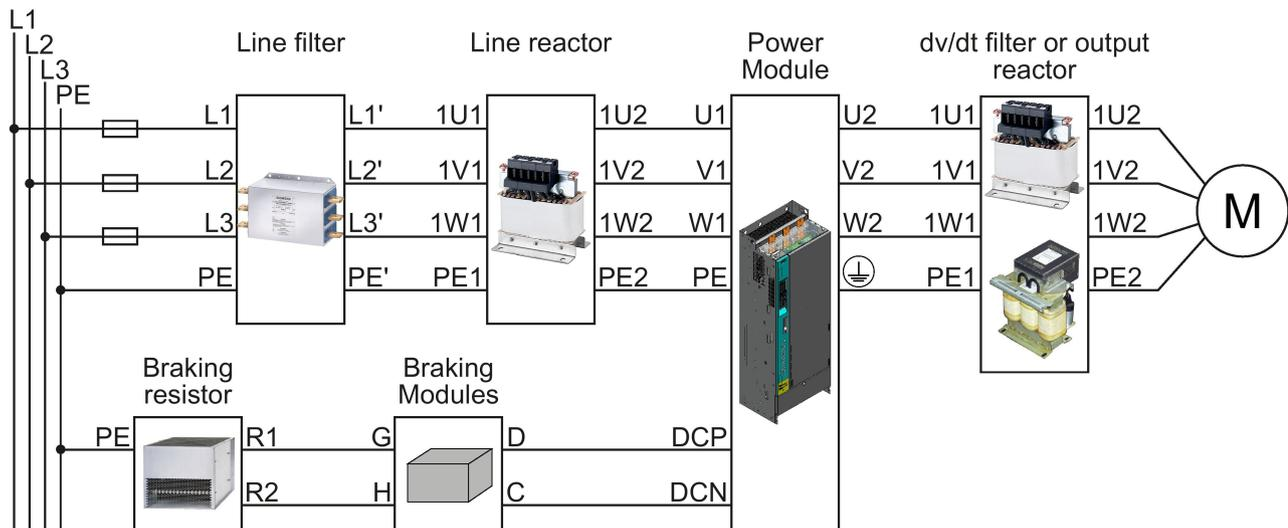
Figure 4-16 Connecting the PM330 Power Module
