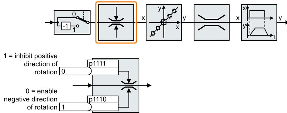
If you want to permanently enable the negative direction of rotation, then set parameter p1110 to 0.
