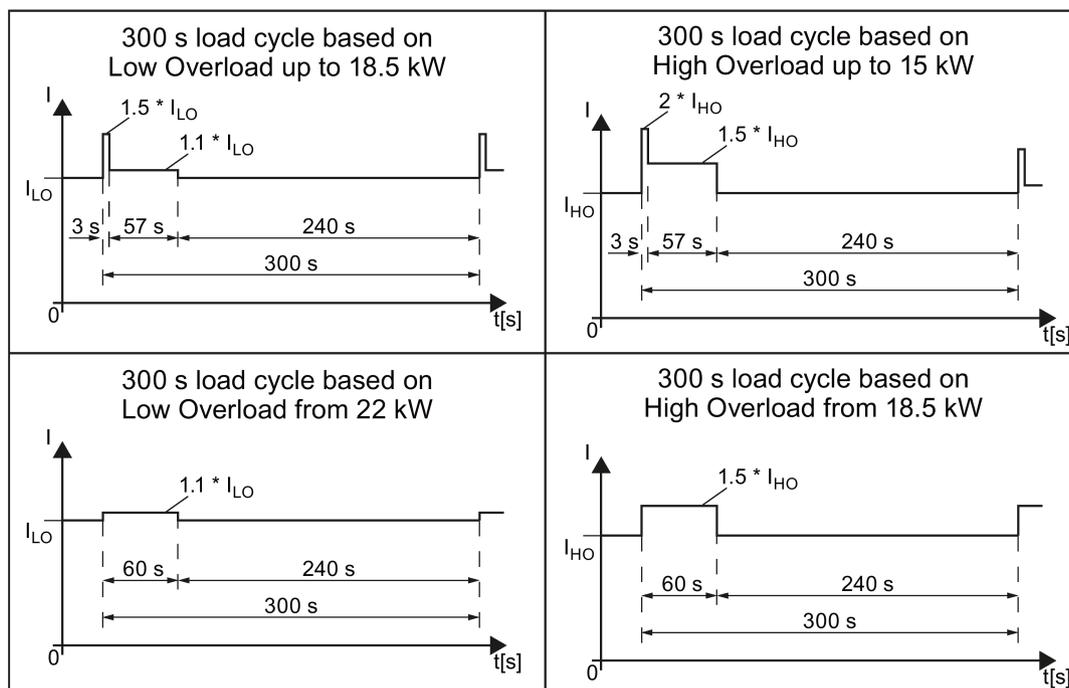
Figure 10-2 Duty cycles, "High Overload" and "Low Overload"
