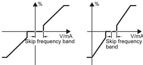
Interferences in the cable can corrupt small signals of a few millivolts. To be able to enter a setpoint of exactly 0 V via an analog input, you must specify a skip frequency band.
