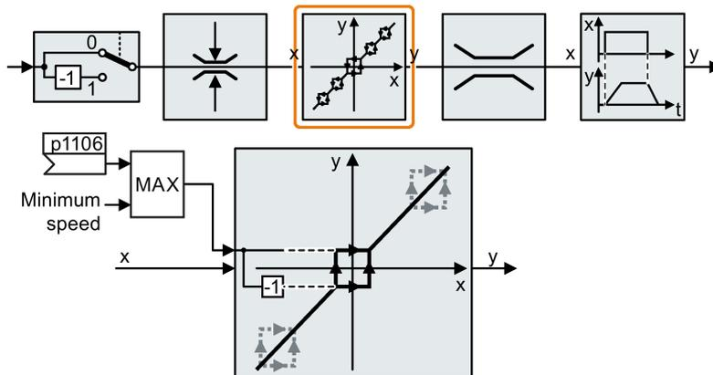
Speeds where the absolute value is less than the minimum speed are only possible during motor operation when accelerating or braking.
