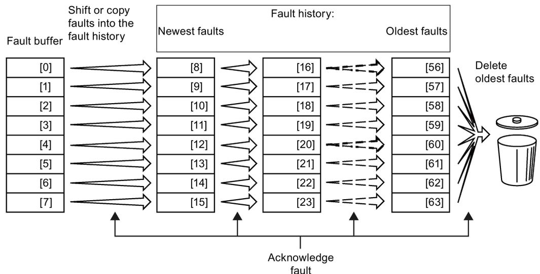
Figure 9-8 Fault history after acknowledging the faults
