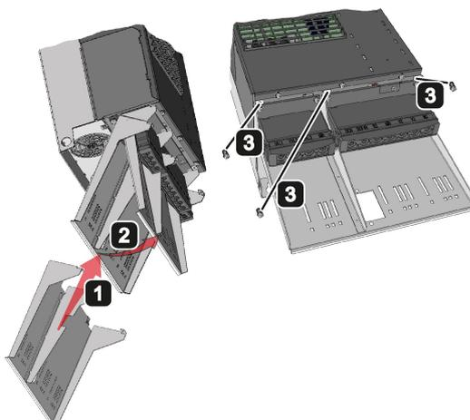
Figure 4-2 Mounting the shield plate, FSD ... PSF
