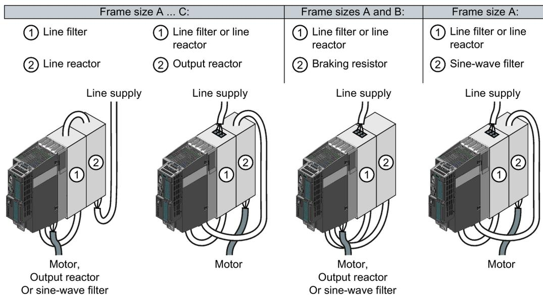
Figure 4-7 Permissible combinations of two base components
