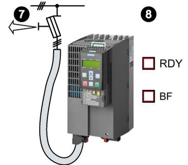
9. Switch on the inverter power supply again.
