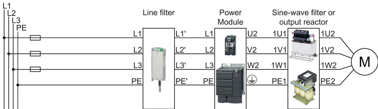
Figure 4-14 Connecting the PM250 Power Module
