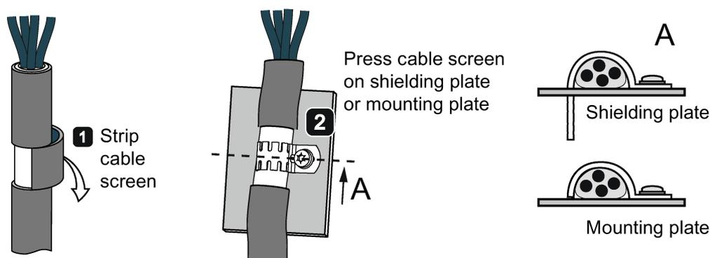
Figure 4-4 Shield connection - detail
