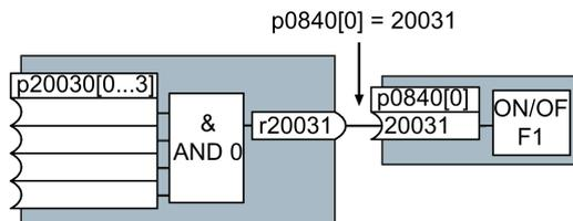
Figure A-8 Interconnecting blocks by setting p0840[0] = 20031
