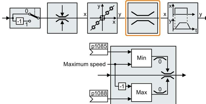
The converter generates a message (fault or alarm) when the maximum speed is exceeded. If you must limit the speed depending on the direction of rotation, then you can define speed limits for each direction.
