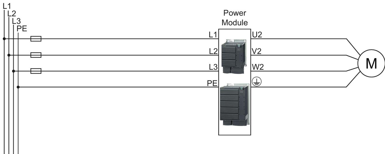
Figure 4-15 Connecting the PM260 Power Module
