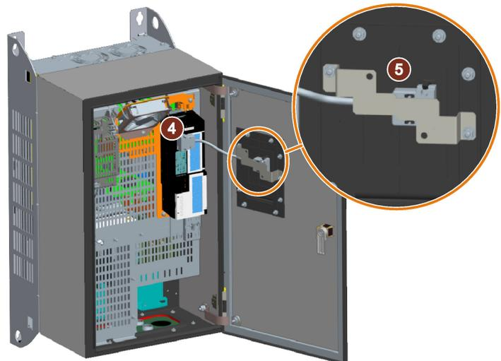
■ You have installed a Control Unit in an IP55 Power Module FSD ... FSF.
