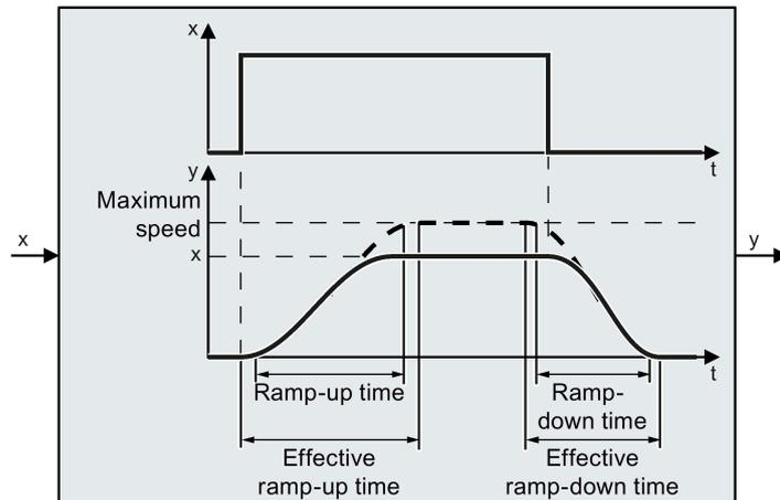
Initial and final rounding permit smooth, jerk-free acceleration and braking.
