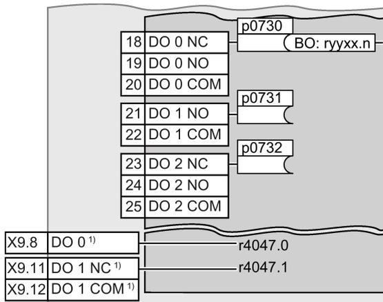
To change the function of a digital output, you must interconnect the digital output with a binector output of your choice.
