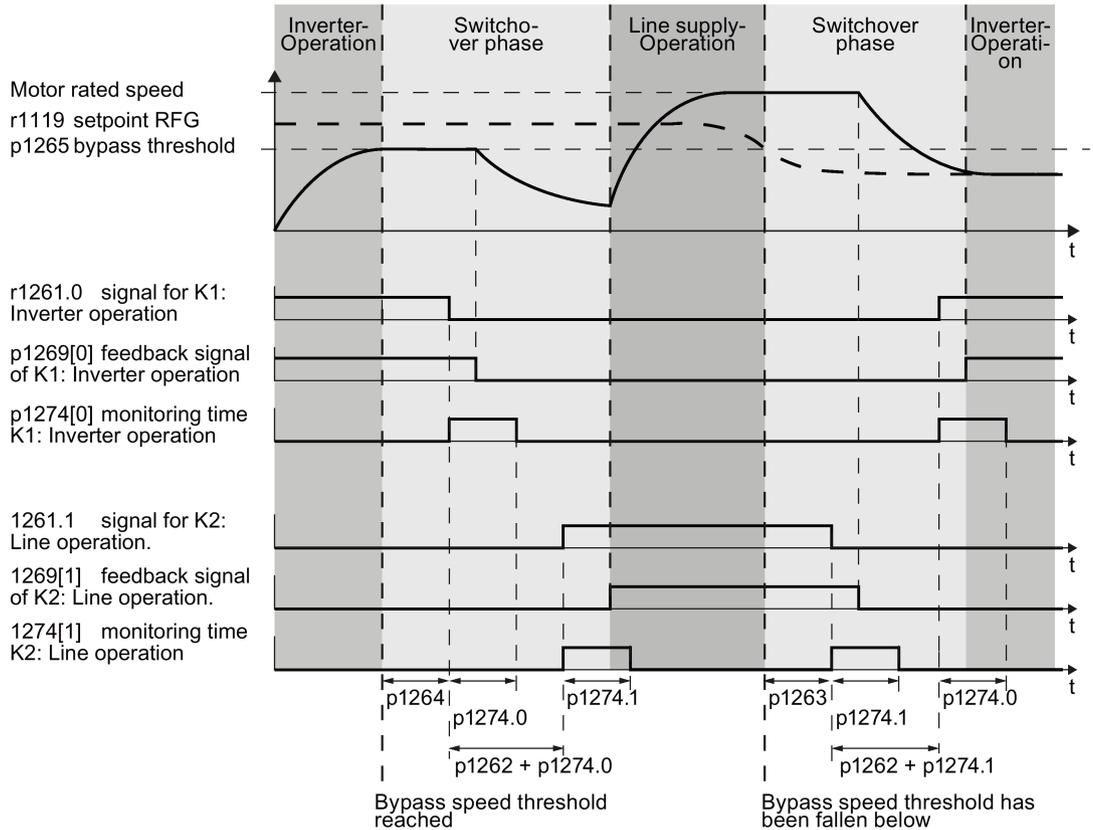
Figure 6-49 Switchover behavior from inverter to line operation dependent on the speed
