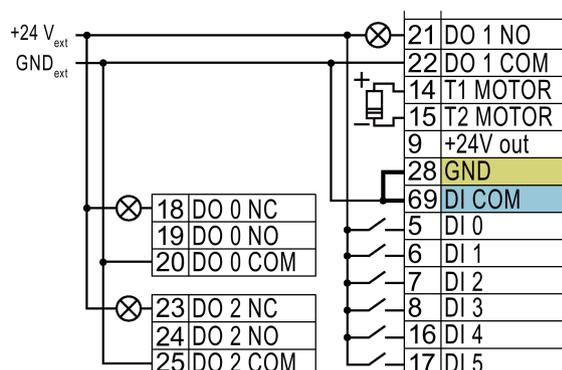
You must remove the jumper between terminals 28 and 69 if it is necessary to have electrical isolation between the external power supply and the internal inverter power supply.
