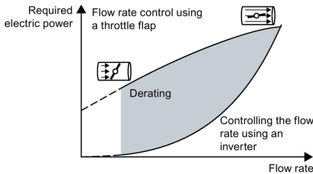
The converter calculates the energy saving from the flow characteristic associated with a mechanical flow control and the measured electric power that is drawn.
