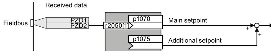
Figure 6-22 Fieldbus as setpoint source
