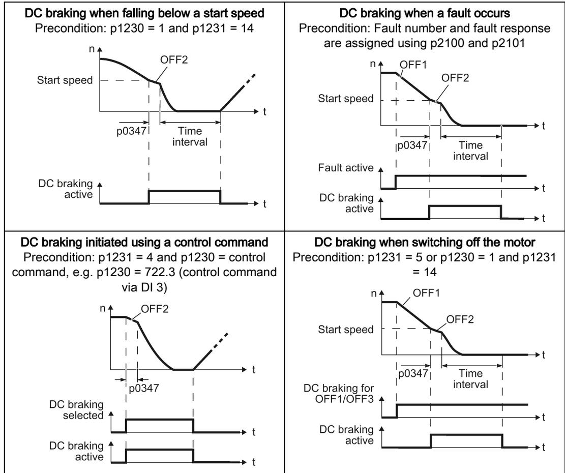
**DC braking when falling below a starting speed**
