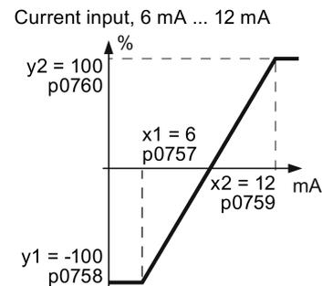
Set the following parameters to set the analog input as current input with monitoring:
