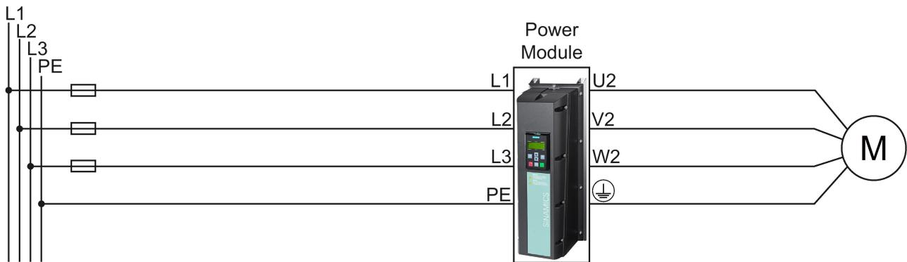
Figure 4-12 Connecting the PM230 IP55 Power Module
