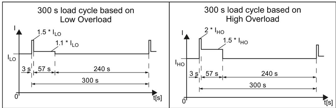
Figure 10-5 Load cycles "Low Overload" and "High Overload"
