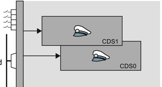
You select the command data set using parameter p0810. To do this, you must interconnect parameter p0810 with a control command of your choice, e.g. a digital input.
