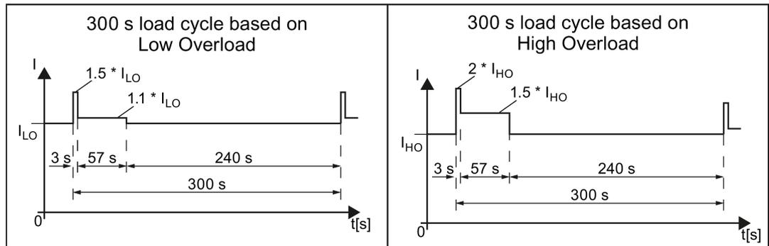
Figure 10-6 Load cycles "Low Overload" and "High Overload"
