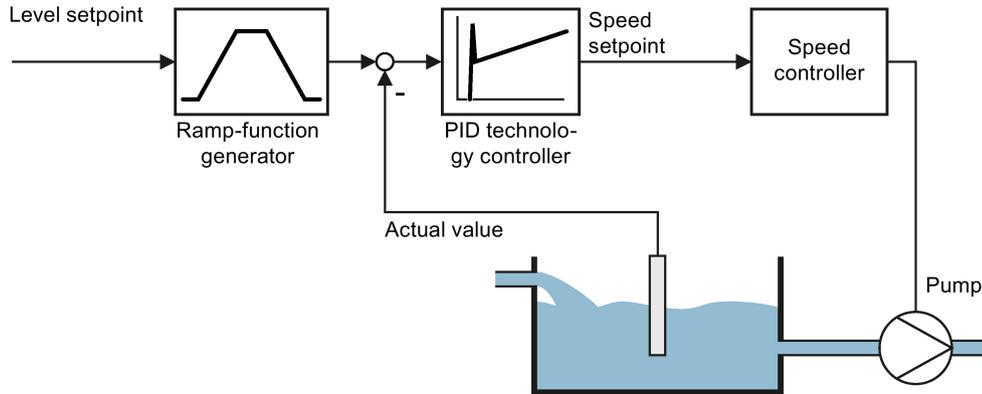
Figure 6-42 Example: Technology controller as a level controller
