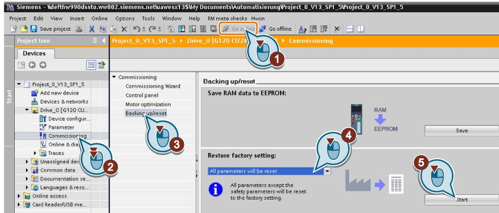
6. Wait until the inverter has been reset to the factory setting.
