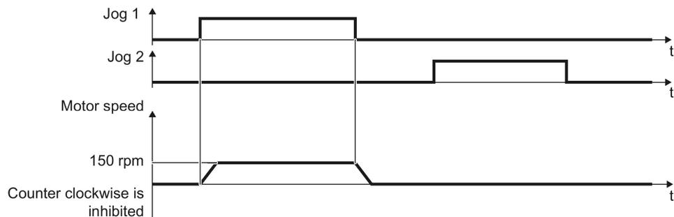
Figure 5-2 Jogging the motor in the factory setting
