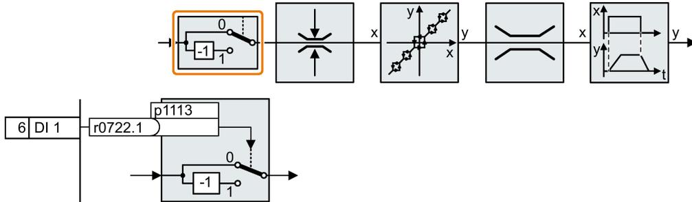
In order to invert the setpoint through the digital input DI 1, connect the parameter p1113 with a binary signal, e.g. the digital input 1.
