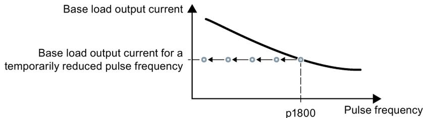
Figure 6-34 Derating characteristic and base load output current for overload
