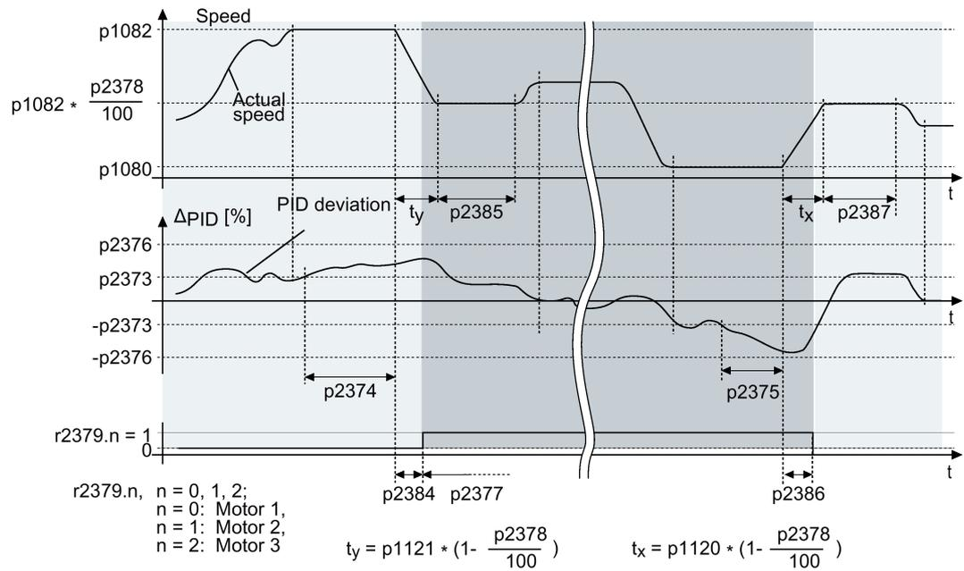
Figure 6-50 Conditions for activating/deactivating an uncontrolled motor
