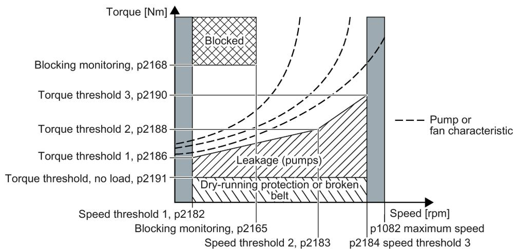
If the torque or the speed moves, for longer than the time set in p2192, in the ranges of blockage, leakage or dry running protection/belt breakage, then the response defined in p2181 is realized.
