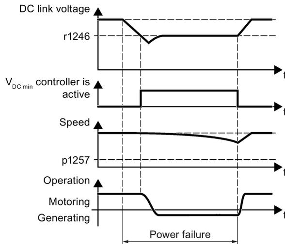
Figure 6-40 Principle mode of operation of kinetic buffering
