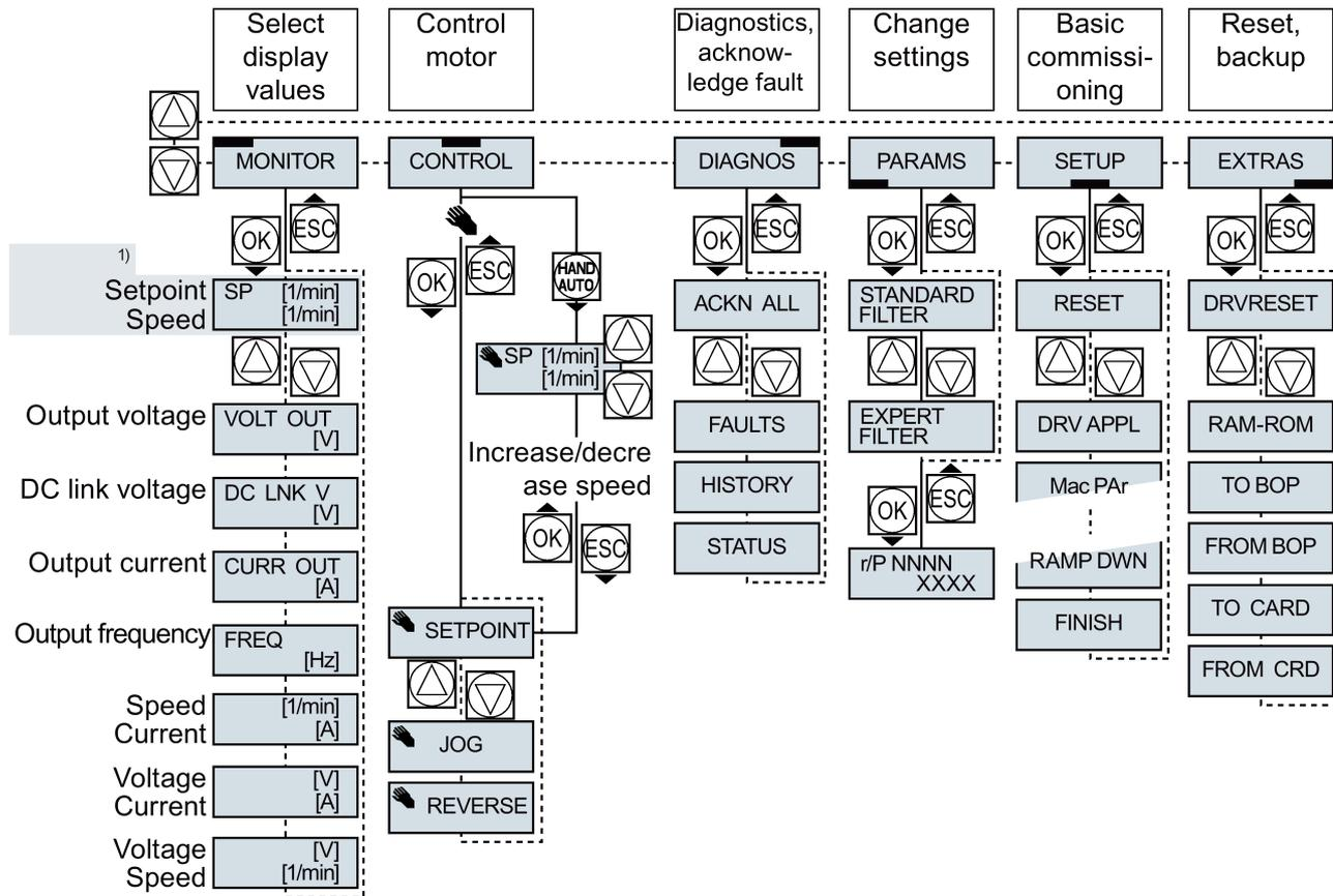
1) Status display once the power supply for the inverter has been switched on.
