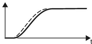
The speed setpoint (broken line) increases with the set ramp-up time and rounding.
