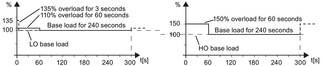
Figure 10-7 Load cycles, "Low Overload" and "High Overload"
