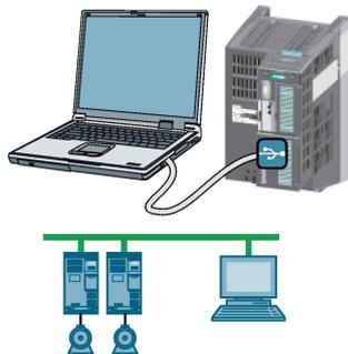
You can access the inverter with STARTER or Startdrive either via a USB connection or via the fieldbus.
