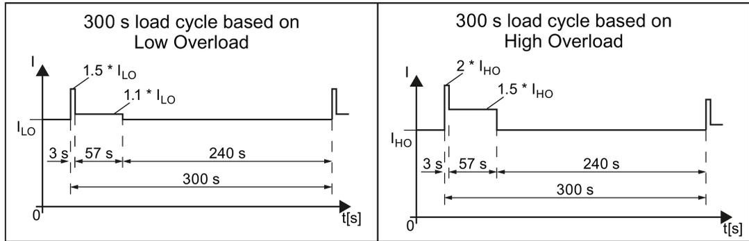
Figure 10-3 "Low Overload" and "High Overload" load cycles
