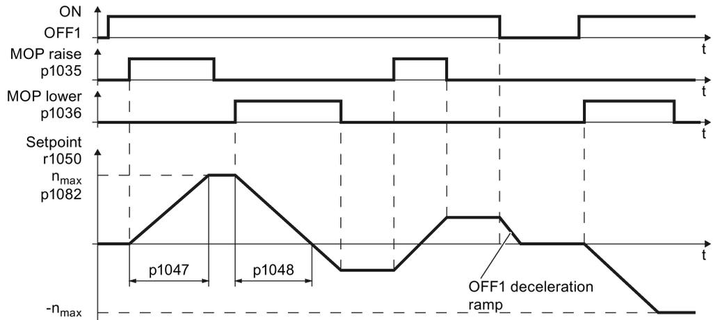
Figure 6-24 Function chart of the motorized potentiometer
