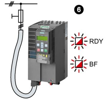
7. Switch off the inverter power supply.
