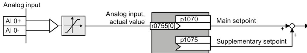
Figure 6-21 Example: Analog input 0 as setpoint source
