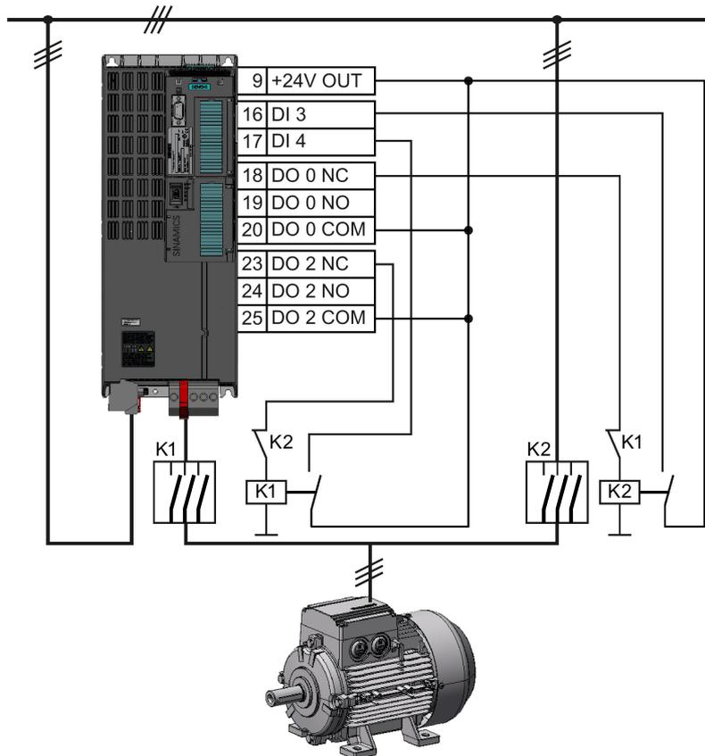
Figure 6-47 Bypass circuit for control using the inverter
