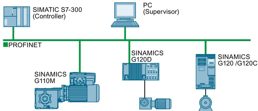
In PROFINET IO operation, the inverter supports the following functions:
