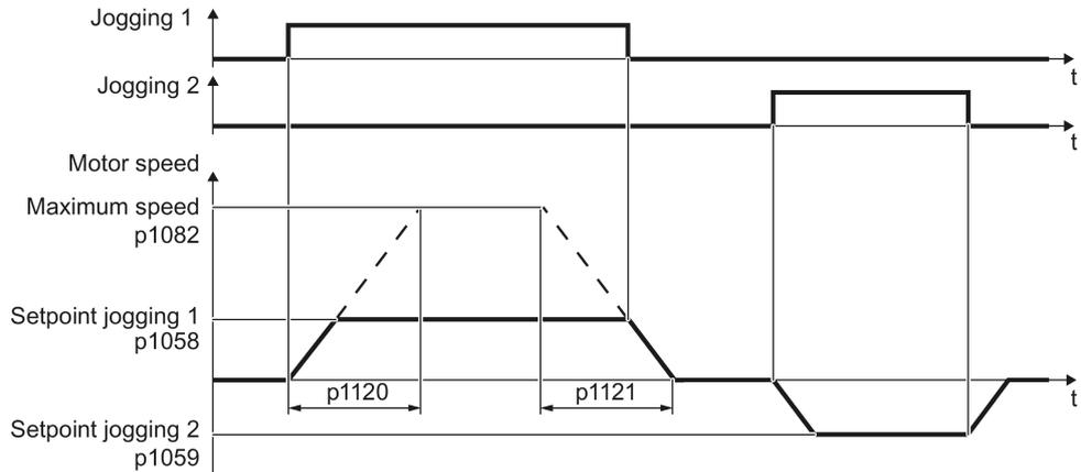
Figure 6-11 Behavior of the motor when "jogging"
