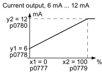
Set the following parameters to set the characteristic to match the example:
