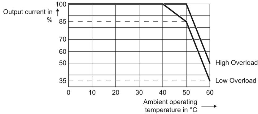
The Control Unit and operator panel can restrict the maximum permissible operating ambient temperature of the Power Module.
