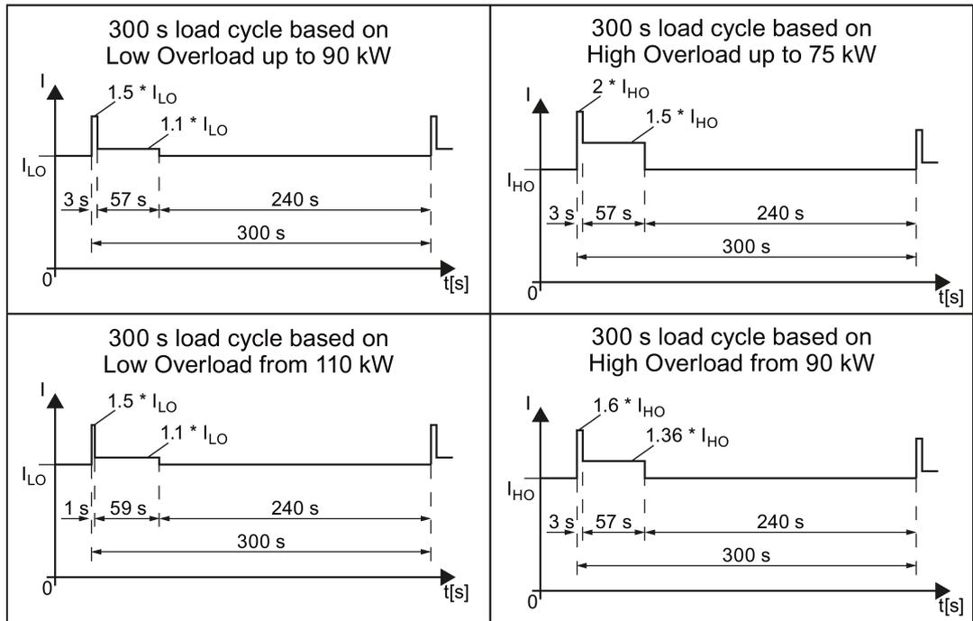
Figure 10-4 "High Overload" and "Low Overload" load cycles
