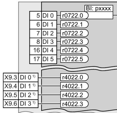
To change the function of a digital input, you must interconnect the status parameter of the digital input with a binector input of your choice.
