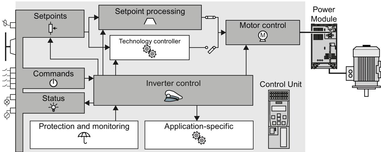
Figure 6-1 Overview of inverter functions
