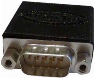
Figure 3-1 Distance connector for the connection between a Control Unit and Operator panel
