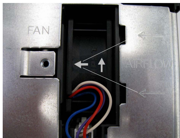
Figure 13-1 Arrows on the fan for the air flow direction
