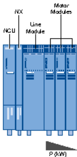
Figure 4-12 NX between NCU and Line Module
