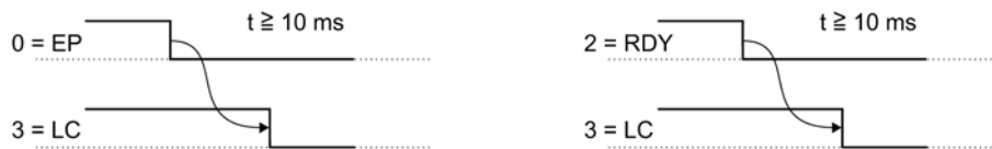
Figure 6-7 Line contactor control signal chart
