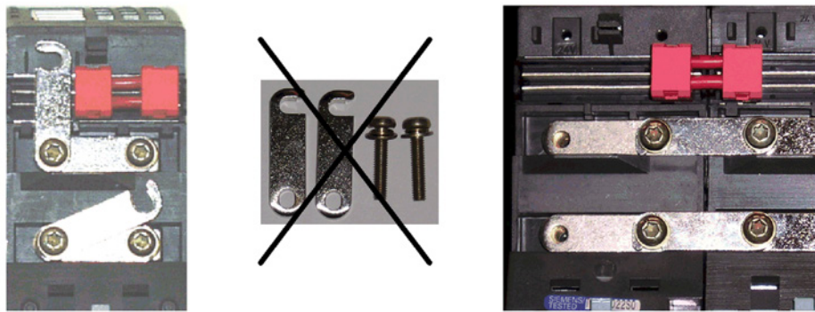
Figure 4-1 Removal of the DC link bridge
