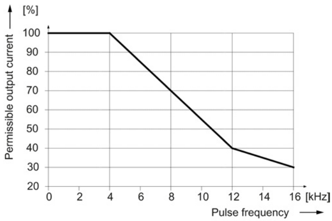
Figure 8-161 Output current as a function of the pulse frequency for 200 A Motor Modules (applies from order number 6SL312x-1TE32-0AA4)
