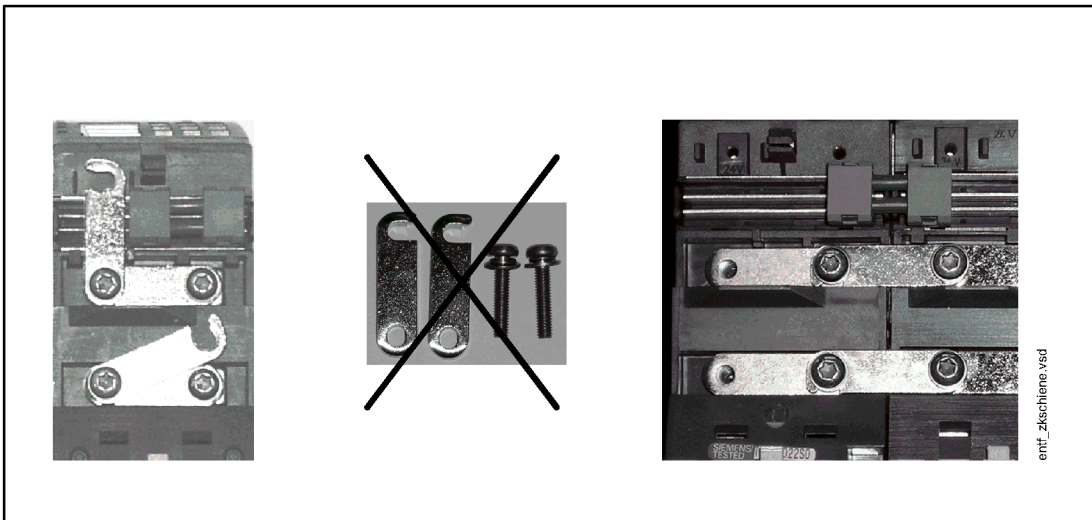
Figure 12-3 Removing the DC link bridges (multi-tier configuration)
