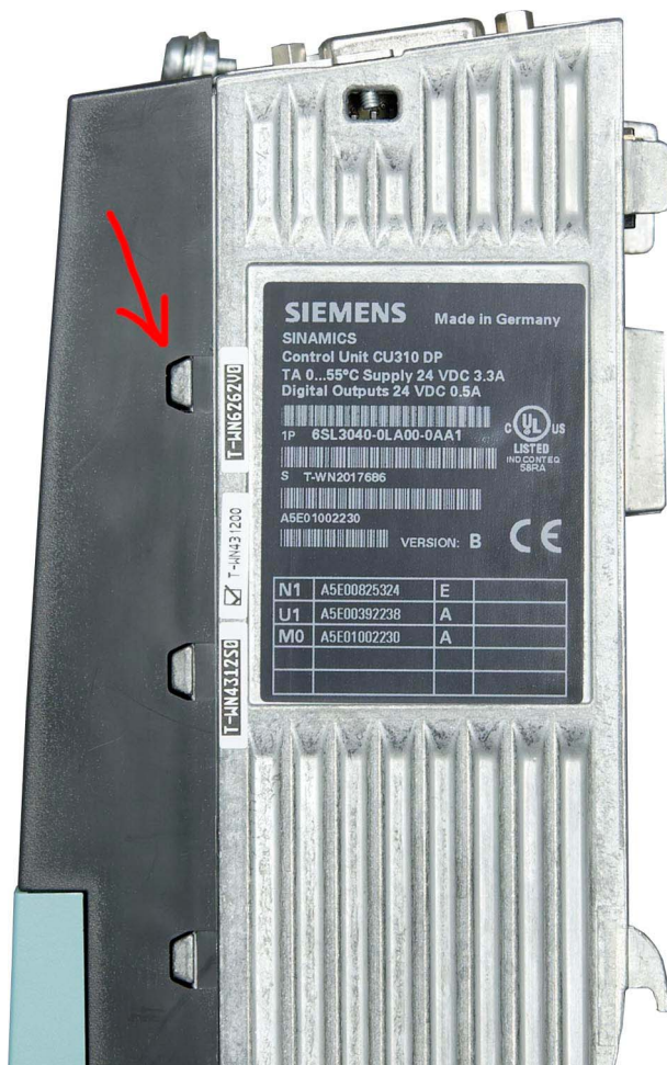
Figure 11-1 Lateral snap hooks on a CU310 DP
