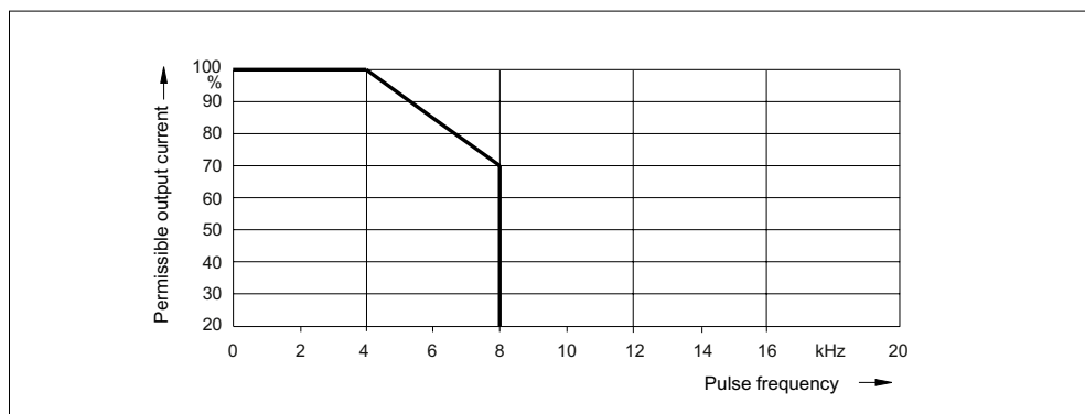
Figure 3-26 Frame size FSF: Output current as a function of the pulse frequency
