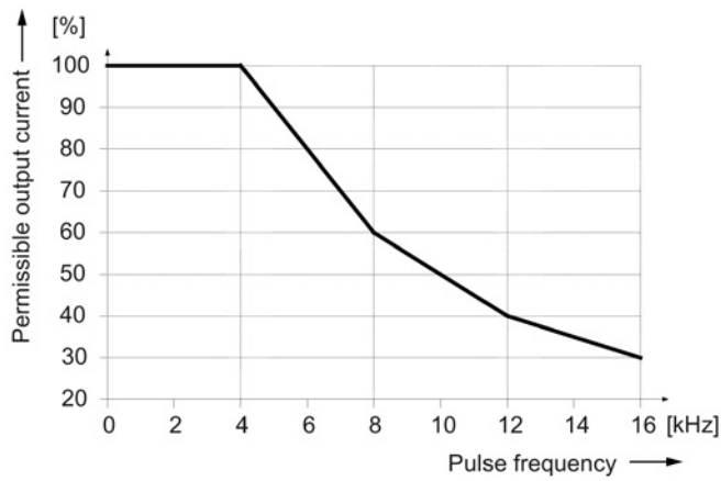
Figure 6-99 Output current as a function of the pulse frequency
