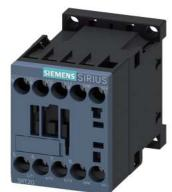
power contactor, AC-3e/AC-3, 7 A, 3 kW / 400 V, 3-pole, 110 V DC, auxiliary contacts: 1 NC, screw terminal
