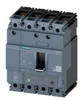
circuit breaker 3VA1 IEC frame 160 breaking capacity class S Icu=36kA @ 415V 4-pole, line protection TM240, ATAM, In=100A overload protection Ir=70A...100A short-circuit protection Ii=5...10 x In N conductor protection 100% nut keeper kit
