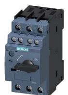
Circuit breaker size S0 for motor protection, CLASS 10 A-release 1.4...2 A N-release 26 A screw terminal Standard switching capacity with transverse auxiliary switches 1 NO+1 NC  $\,$
