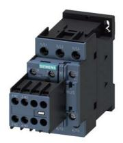
power contactor, AC-3e/AC-3, 32 A, 15 kW / 400 V, 3-pole, 110 V AC, 50 Hz, auxiliary contacts: 2 NO + 2 NC, screw terminal, removable auxiliary switch
