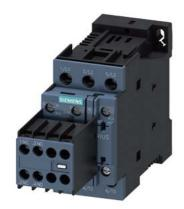
power contactor, AC-3e/AC-3, 32 A, 15 kW / 400 V, 3-pole, 110 V DC, auxiliary contacts: 2 NO + 2 NC, screw terminal, removable auxiliary switch
