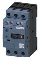
Circuit breaker size S00 for motor protection, CLASS 10 A-release 1.4...2 A N-release 26 A Screw terminal Standard switching capacity with transverse auxiliary switch 1 NO+1 NC  $\,$
