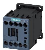
power contactor, AC-3e/AC-3, 7 A, 3 kW / 400 V, 3-pole, 110 V AC, 50/60 Hz, auxiliary contacts: 1 NC, screw terminal
