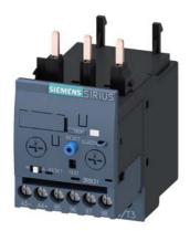
Overload relay 6...25 A Electronic For motor protection Size S0, Class 5...30 Contactor mounting Main circuit: Screw Auxiliary circuit: Screw Manual-Automatic-Reset Internal ground fault detection
